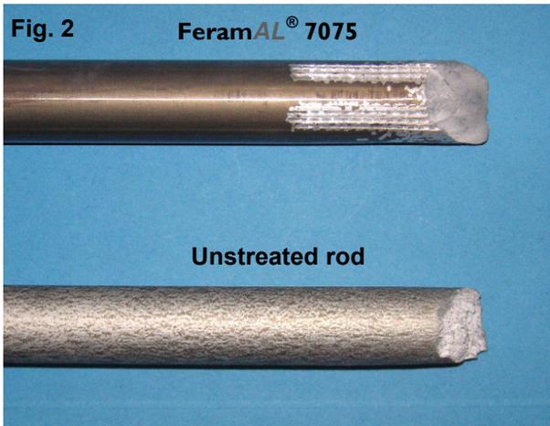
Figure 2 shows the result of a pulling test on an untreated rod and a **FeramAL® 7075** rod.
